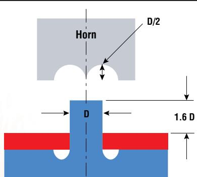
**III** Plexiglas acrylic resins may be heat staked for assembly to materials that cannot be welded, e.g. metals and crystalline polymers. Staking is readily accomplished using heat or ultrasonic energy.
